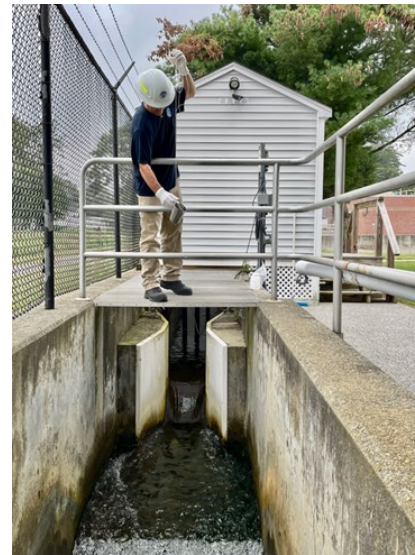
Figure 2: Collecting PFAS samples at the Clinton Wastewater Treatment
